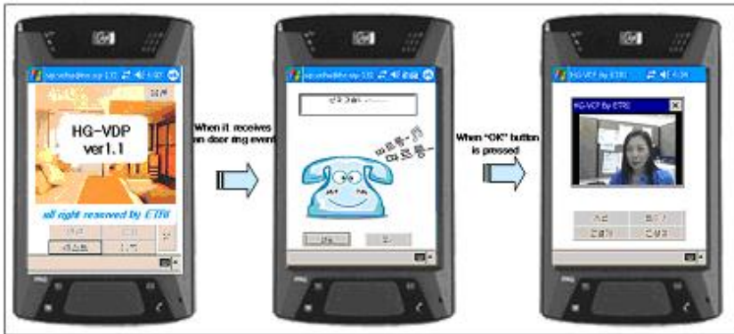
Fig. 5. The User Terminal Agent application with a PDA, for door ring event notification and communication
